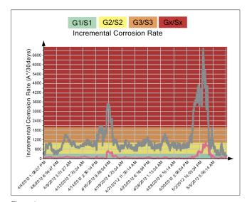
Chemical media change clearly indicated increased levels of corrosion in real-time from SAAFShield® Detecting Unit
